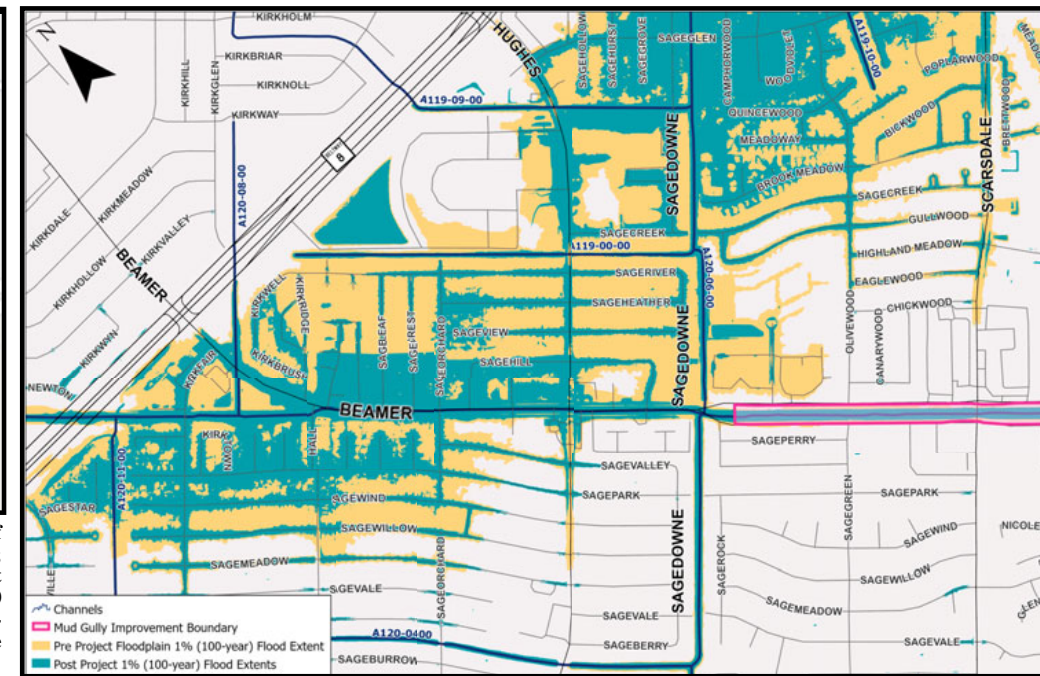
Shown is the area of the Beamer Road ditch which will undergo construction the end of 2020 or the early part of 2021. Phase 1 is from Sagerock Drive to Scarsdale Boulevard; Phase 2 is from Scarsdale to Astoria Boulevard and Phase 3 is from Astoria to just past the turn in the Beamer ditch project. The diagram at right shows the approximate 400 homes which will be removed from the 100-year-flood plain after the two-year construction project. While the entire gold and teal areas are currently in the flood plain, the planned improvements will remove the teal-colored area from the 100-year flood plain.
